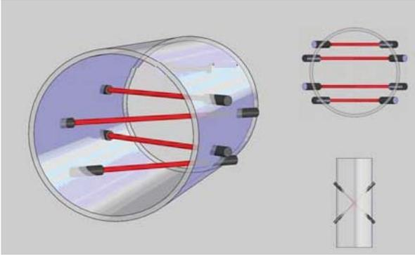
Figure 1. Transducer position in a 4-path USM
